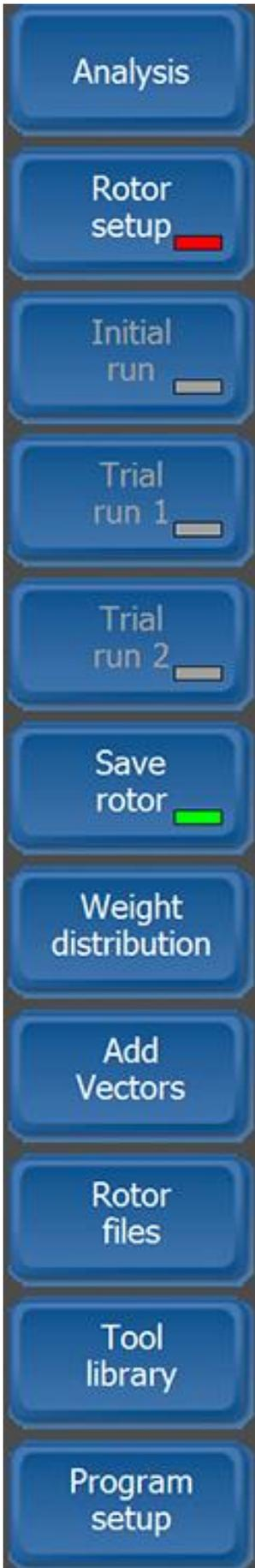
**Analysis** Allows to measure spectrum before and after balancing and do a resonance test
