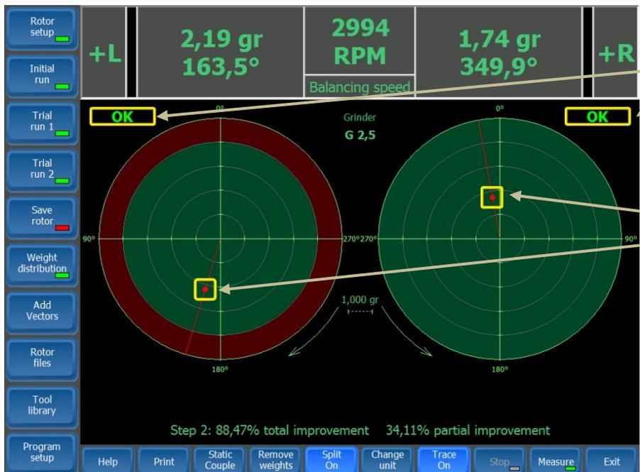
In this case, vibrations in both planes are within limits. This is acknowledged with a green "OK" for each plane.
